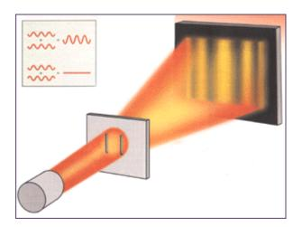
Thomas Young's experiment with two narrow slits inserted between the light source (here a laser) and the detector (here a screen). Waves emerging from one slit are superimposed on waves from the other slit, producing the observed interference pattern with alternate dark and bright lines on the screen.
